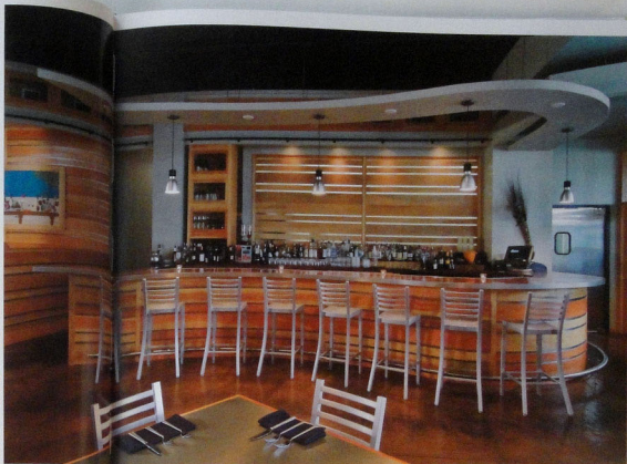
ABOVE: The curving interior bar is the central gathering space and heart of DUCE. The base alternates douglas fir bands with strips of stainless steel and the top is cast-in-place concrete finished to match the floors. The douglas fir screen behind the bar is actually in front of a glass window that looks into the kitchen. A curving soffit overhead reinforces the shape of the bar. OPPOSITE: The facade incorporates the standard shopping center tower element and finishes with the signature DUCE wood and glass storefront.
